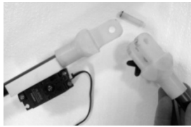
Figure 14. Constructed elbow joint.
