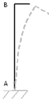
Figure 6: Deflected shape of column corresponding to the standard approximate analysis.
