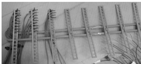
Figure 9. Thermocouple tree with thermocouples during assembly.
