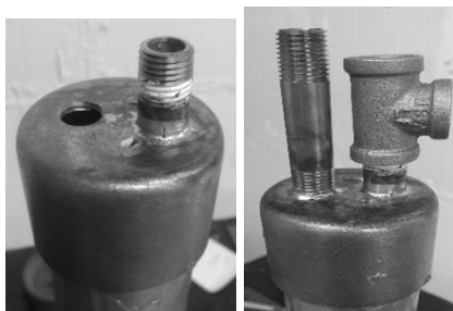
Figure 8. (Left) 2-in copper cap with 1/4-in npt nipple. (Right) Soldered 1/4-in npt nipple fittings on top 2-in end cap.
