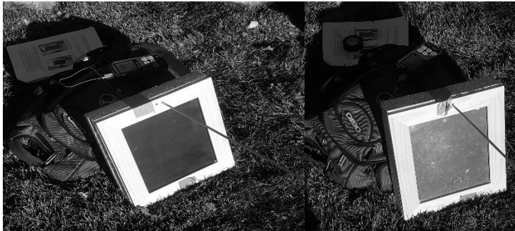
Figure 2. (Left) Picture of experimental setup with black painted surface facing out. (Right) Picture of experimental setup with the aluminum surface facing out.
