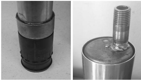
Figure 7. (Left) Copper cap and brass pipe held vertical. (Right) 1 7/8-in pipe with 1 1/2-in copper end cap concentric and flush.
