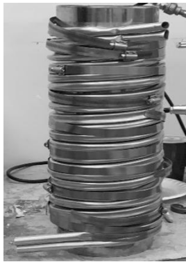
Figure 1: Copper vessel with copper tubing wrapped in a helical arrangement.
