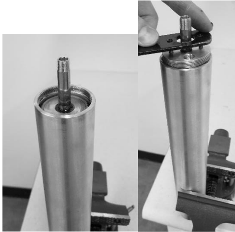
Figure 6. Gluing the second cap into the diathermometer.
