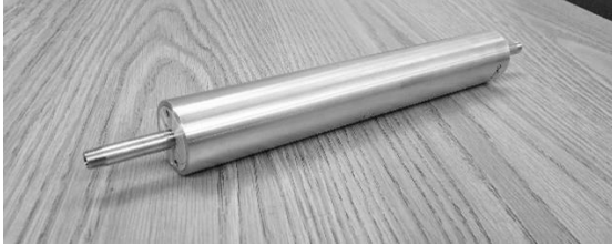
Figure 3. Caps and nipples glued into small tube.
