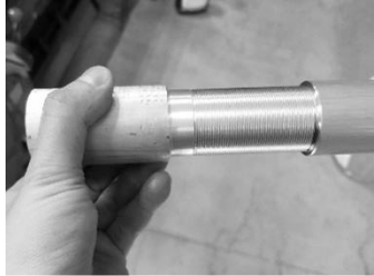
Figure 2. Threading each tube to fit the threaded bar stock.
