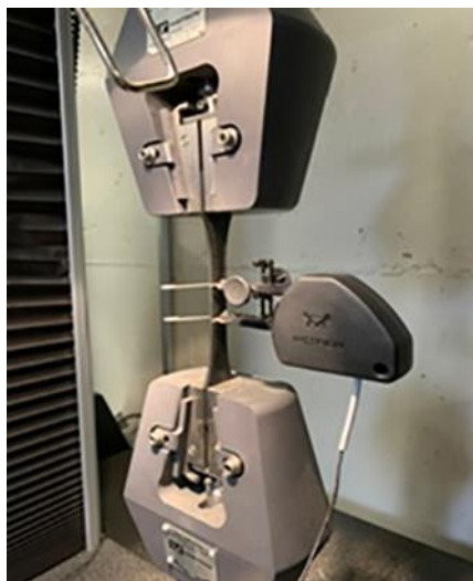
Figure 4. PLA sample in Instron 5582 testing machine.
