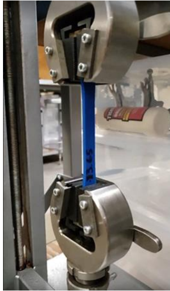
Figure 7. Tension bar loaded into the universal testing machine.
