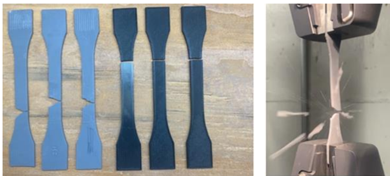
Figure 9. (Left) Image of the test samples after testing. (Right) Image of resin sample fracture.
