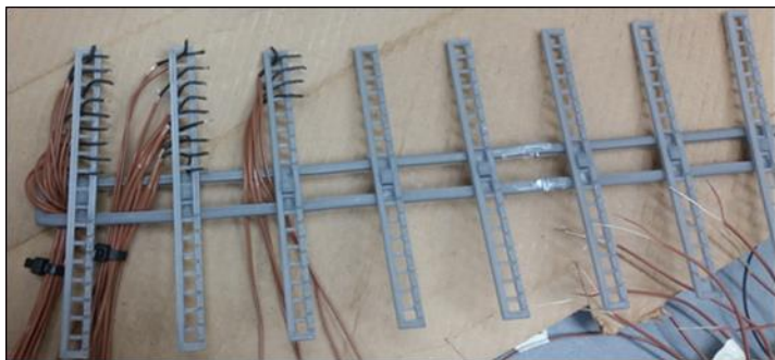
Figure 2. Thermocouple tree used to measure water temperature.
