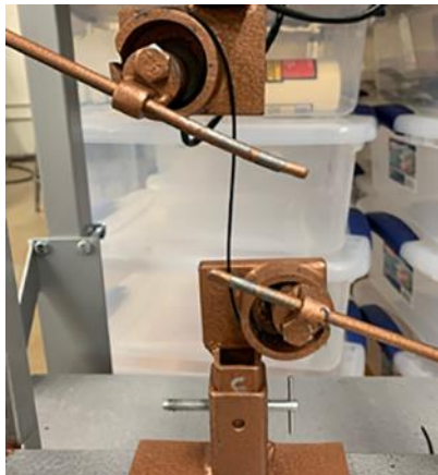
Figure 6. PLA wire sample set up for testing in grips.
