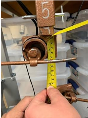
Figure 5. Setting initial length of the PLA wire sample test to 5".
