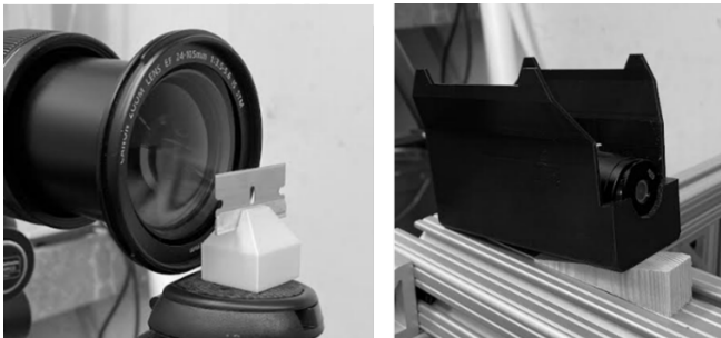
Figure A-4. Schlieren components: razor blade (left) and flashlight (right).
