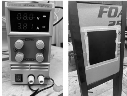
Figure A-2. Power source (left) used for the heated plate in the frame (right).
