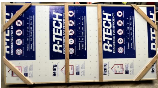
Figure B4. Finished frame with insulation board.
