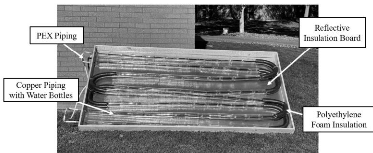
Figure 1. The solar heater apparatus.
