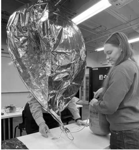
Figure 6. Filling balloon with approximate neck lift attached.
