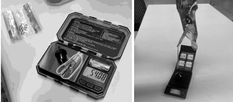
Figure 8. (Left) Taring the system. (Right) Precise neck lift measurement.
