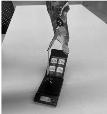
Figure 3. Precise neck lift measurement.
